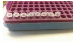
Fig 1- Eight PCR Tubes prepared for gradient thermal cycling- solution previously prepared
